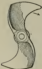
484. TYPES OF PROPELLERS. The Hirsh propeller. The generating line is the segment of an Archimedes spiral, with the leading edge of the blades curved forward, face of the blades curved with increasing pitch.
